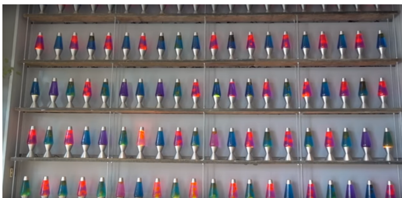
Figure 1.1: A wall full of lava lamps, used to generate random numbers. Screenshot taken from www.youtube.com/watch?v=1cUUfMe0ijg at 2:53.
